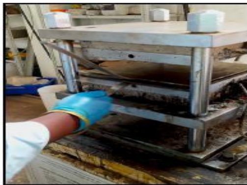
Fig. 12. Demolding of the composite specimen after compression molding using a hydraulic press.
