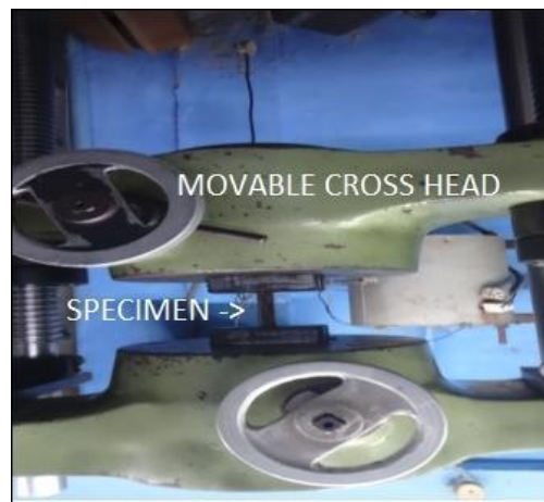
Fig. 13. Tensile Testing: This represents the tensile strength test performed on the composite specimen.
