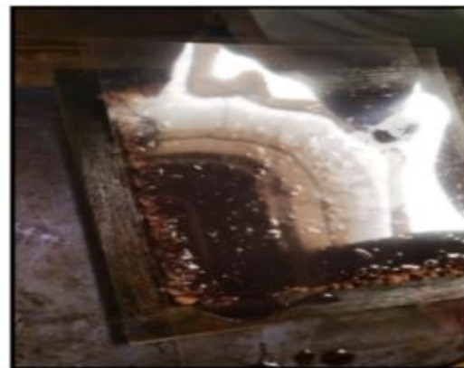
Fig. 10. Addition of a release film over the rein-coated fiber mat.
