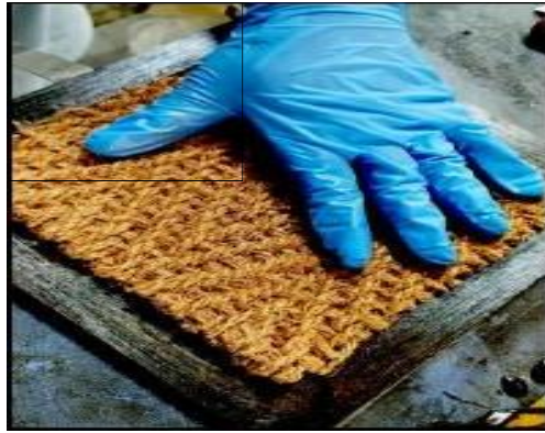
Fig.7. Placement of interlocked coir fiber mat inside the mould.
