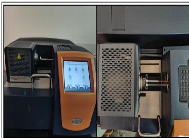
Fig. 16. Thermo Gravimetric Analyser (TGA) Setup
