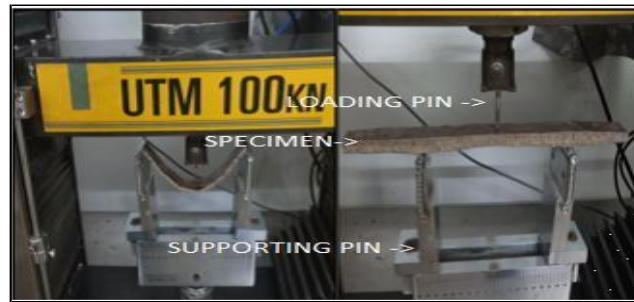
Fig. 14. Flexural Testing: Corresponds to the three-point bending test used to evaluate the flexural strength.
