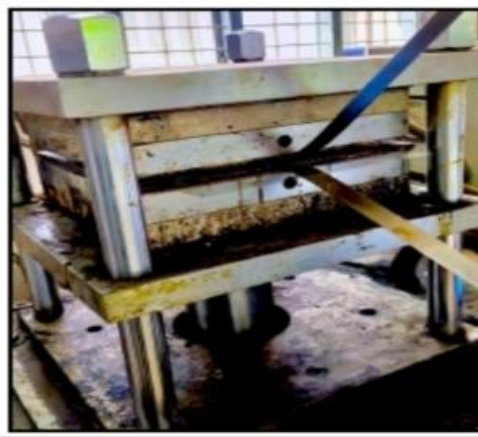
Fig.11. Compression molding setup with a hydraulic press applying pressure.
