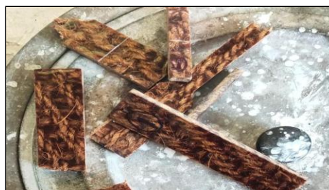
Fig. 18. Tested Interlocked fiber composite material
