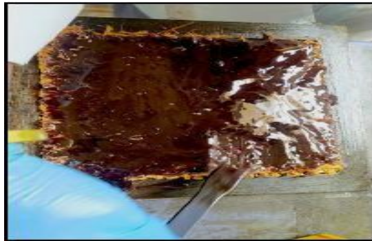
Fig. 9. Spreading the resin uniformly over the coir mat.
