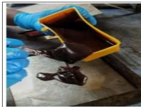
Fig. 6. Spreading the resin evenly inside the mould before fiber placement.
