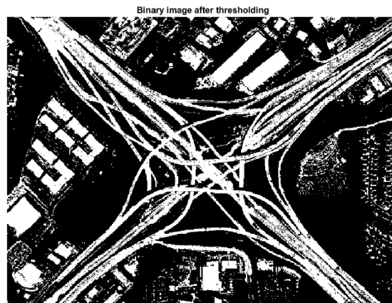
Figure 5.8 Pre-Processing- Binary Image after Thresholding
