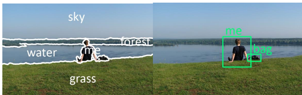
Figure 4.1: Semantic Segmentation v/s Object Detection
